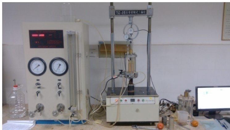
Figure 3. TSZ-3 strain-controlled triaxial tester.
