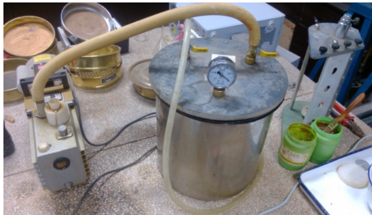
Figure 4. BGH vacuum saturator.
