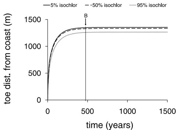
**Figure 2.** Example of time-marching a dispersive interface simulation to steady state conditions (parameter set 1). The transient movements of the 5%, 50%, and 95% seawater isochlors along the aquifer base are displayed. *B* is the time at which the toe rate of change falls below 0.1% of its rate of change during the first year.
