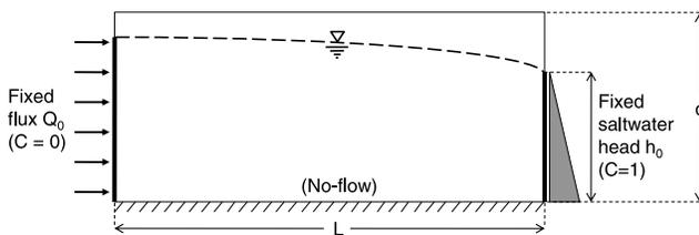
**Figure 1.** Schematic conceptual model of an idealized coastal aquifer system. The concentration of inflows ( $Q_0$ ) through the inland boundary is  $C = 0$ , while ocean boundary inflows occur at seawater concentration ( $C = 1$ ).
