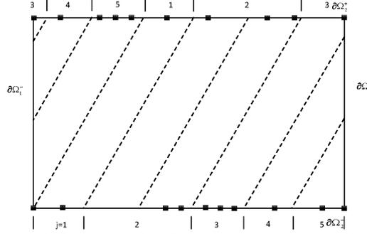
Fig. 3 Tessellation BC for an oblique angle. Black squares symbolize nodes. Dashed lines show a preliminary division of the upper and the lower boundary into integration zones along  $m = 2$ . Zones 1~5 are the final division to ensure every integration zone possesses at least one node per side.
