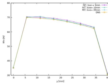
Fig. 9 Horizontal reaction forces along the right edge under tension.
