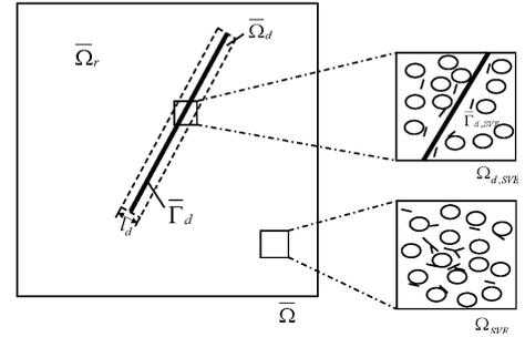
Fig. 2 Dividing the macroscopic domain into two parts,  $\bar{\Omega}_r$  and  $\bar{\Omega}_d$  (left). Each has a characteristic microstructure. A SVE is experiencing material softening (right top) and a SVE is in a state prior to loss of stability (right below).
