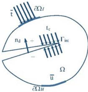
Fig. 1 A 2D solid with a cohesive crack.
