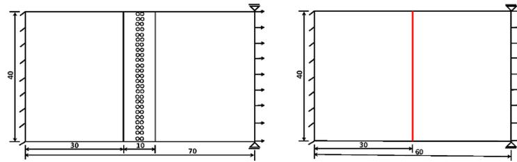
Fig. 4 Geometry of the specimen for the benchmark problem 4.1 (all units in mm): DNS (left) and macroscale in  $FE^2$  (right). The accumulation of voids represents the softening and the red line indicates a cohesive crack.
