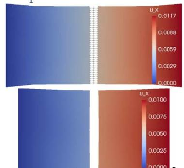
Fig. 7 Horizontal displacements on the deformed configuration ( X 1000): (A) for the DNS and (B) for the macroscale problem ( $FE^2$ ).
