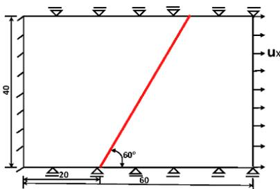
Fig. 8 Geometry of the elastic plate with a cohesive crack (4.2).
