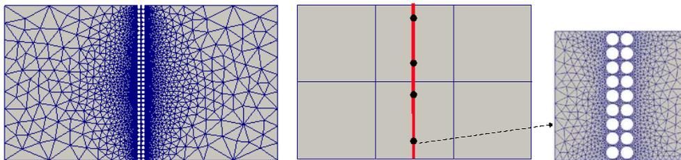
Fig. 5 The discretizations for the DNS (left), the macroscale problem (middle) and the SVE (right) attached to a cohesive zone integration point marked with black dot.
