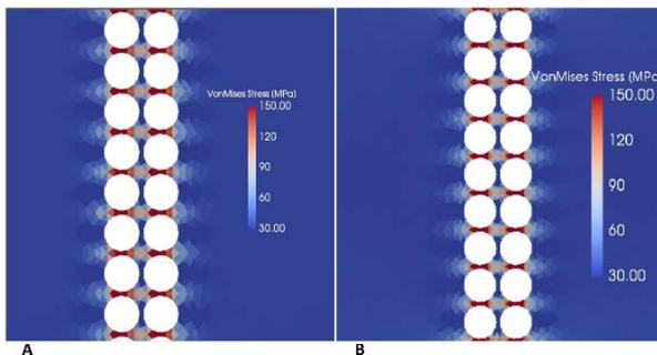
Fig. 6 Von Mises effective stress distribution: (A) on a portion of the voided band in the DNS and (B) on a SVE in the  $FE^2$  simulation
