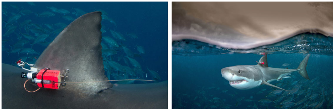
Figure 2: Example of an accelerometer package deployed on a white shark ( Carcharodon carcharias ).
