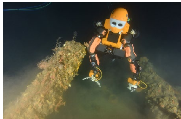
Figure 3. Trials of Techno-Concept's robotic hand off Toulon (F. Osada and T. Seguin, 2014 © DRASSM).
