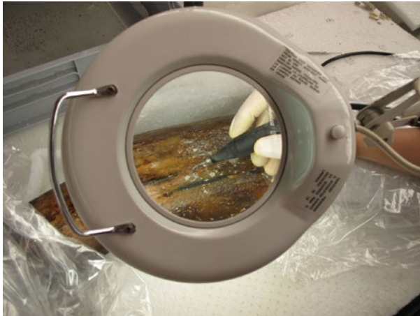
Figure 4. Mechanical cleaning of deposits of biological origin (National Museum of Underwater Archaeology of Cartagena).
