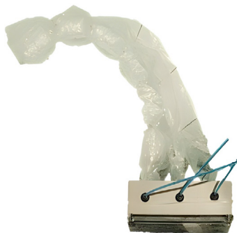
Fig. 6. Robot demonstrating an angle of 65 degrees when inflated to the maximum volume of 3228 ml.
